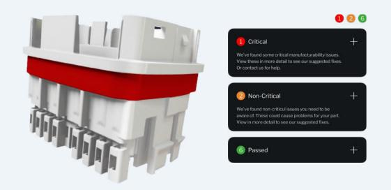
Once you have updated your design to reflect the DFM feedback, we engage in a verification process. Both you and our Fast Radius team will check that the supplier's manufacturability feedback has been implemented and sign off on the DFM report. After this signoff, lead time will be confirmed and the manufacturing process can start.
